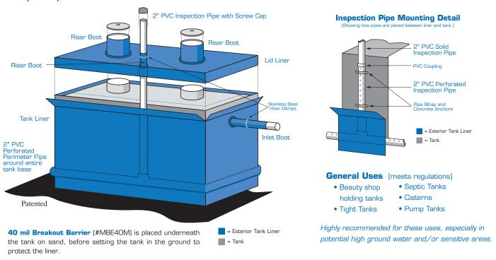
It is recommended you also use the lid liner with manhole riser boot liner which completely encloses the tank for protection of any surface water and dirt getting between the tank and liner.
