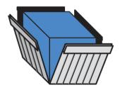
The **Universal Liner**<sup>™</sup> is placed over the core of the mold.
